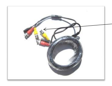
Your cabling has BNC connectors for your video and audio channels. You then have male and female power jacks on each end of your cable. Be sure you install the cable correctly – the female power jack goes to the camera side. There's nothing worse than uninstalling something you just installed because it is backwards – trust us, you will only do it once!
